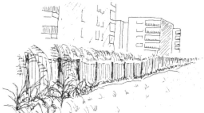
Figure 5-8 Sand Fences trap blowing sand to rebuild frontal dune.
